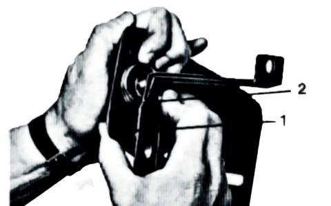
3. Insert bolt (A) into the rudderblade with the washer at the end, so that the bolt projects approx 5-6 mm on the inside of the rudderblade. Fit the appropriate half-bracket to the spring, the bevelled edge turned towards the leg of the spring (see arrow 1), so that the leg of the spring is at the front of the bracket (see arrow 2).
